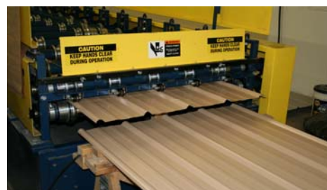
Step 4 Roll Forming Process Finished Panel
